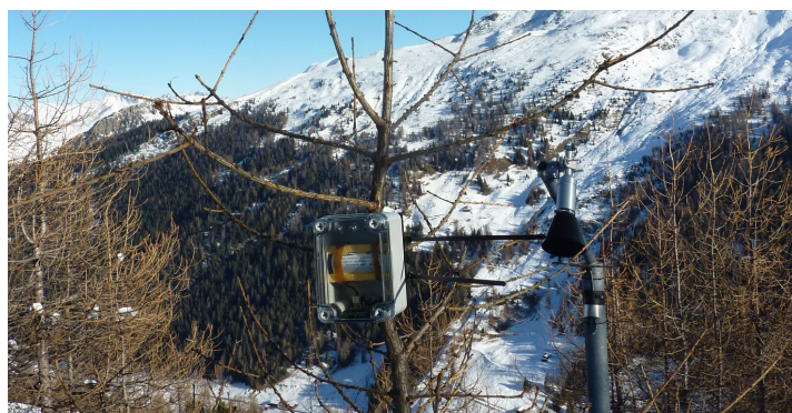
The tree inclination sensor is attached to a larch tree in a waterproof housing.
